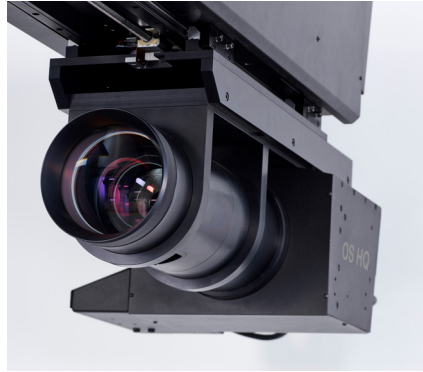
CMOS GigaPixel Camera system with optical zoom
